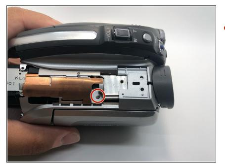
Remove the 5mm screw with your Phillips #0 screwdriver that was previously covered.
