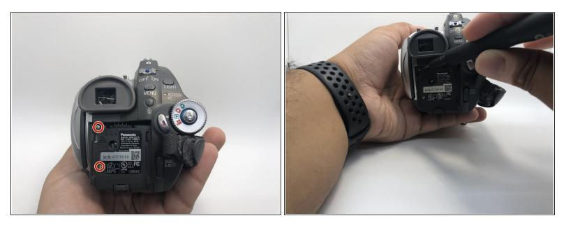
Use your Phillips #0 screwdriver to remove the two 5mm screws on the battery base of the camera.
