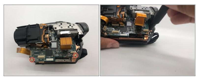
On the motherboard, remove two 5mm screws from the motherboard with your Phillips #0 screwdriver.
