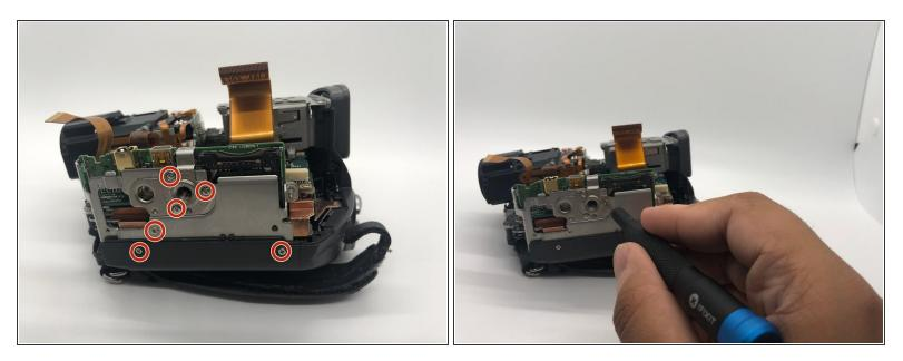
On the bottom side of the camera, remove six 5mm screws with your Phillips #0 screwdriver and the circuit board holder should be free.
