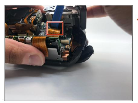
Disconnect another ribbon cable that runs from the motherboard to the bottom of the viewfinder with a plastic opening tool.
