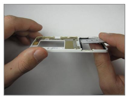
Push the keypad out from the front of the phone and remove it.
