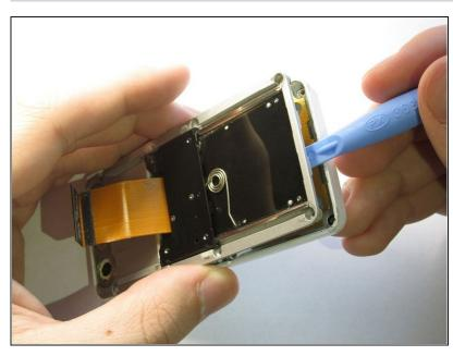
Pry off the back cover from the front of the case using a plastic opening tool.
