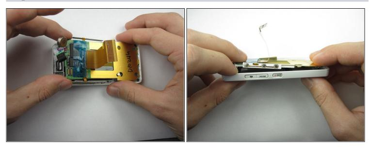
• Starting with the side that has the speaker and receiver, carefully lift the LCD Board out of the case.
