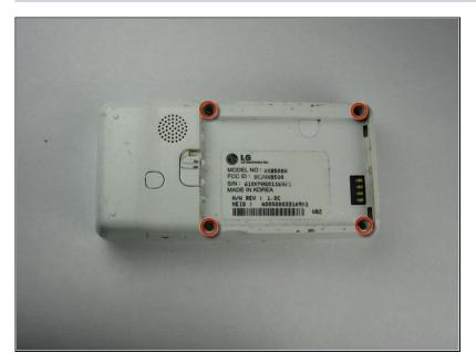
Use a Phillips #00 screwdriver to unscrew the four Phillips #00 screws on the four corners under the battery to unfasten the back case from the phone.
