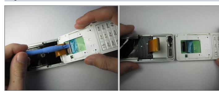
Between the two halves is a ribbon. Use a plastic opening tool to flip up the lock and disconnect it.
