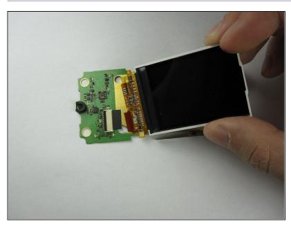
• The LCD screen is no longer connected to the LCD board.
