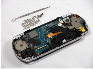
Remove metal shields by gently lifting them with an opening tool.
