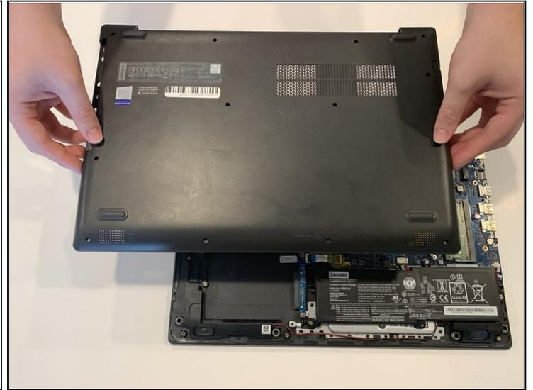
① Make sure that the back panel is completely free from the laptop.
