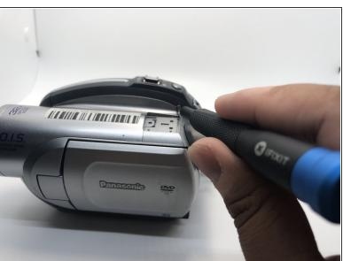
Remove one 5mm screw by using Phillips #0 screwdriver.
