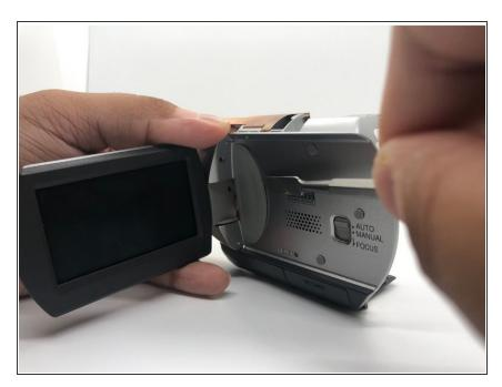
Use a plastic spudger to apply a firm amount of pressure to pry the hinge from the rest of the camera body.
