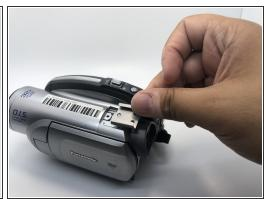
Remove all three 5mm screws from the top of the camera using a Phillips #0 screwdriver.
