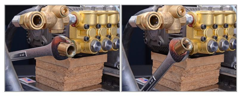
• Use a 1" or large adjustable wrench to loosen and unscrew the pump input elbow.
