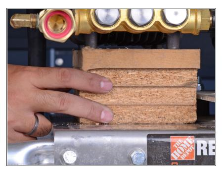
Slide a 3" tall block underneath the pump assembly to help support the pump.
