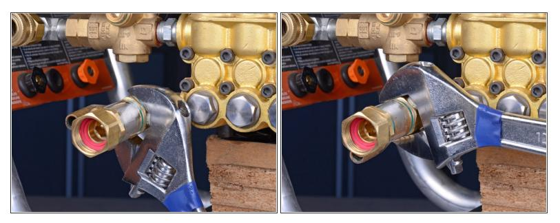
• Use a large adjustable wrench to loosen and unscrew the filter.
