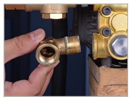
• Remove the input elbow fitting.
