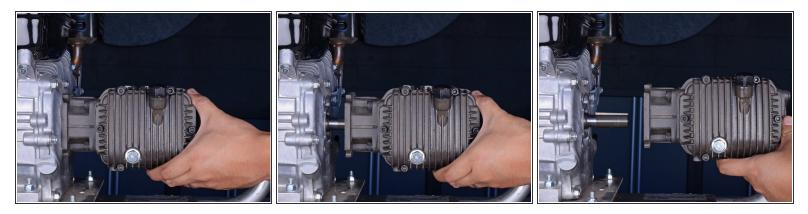
Carefully pull the pump assembly away from the engine until it de-couples from the engine axle.
