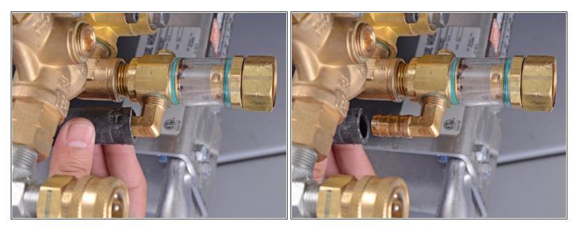
• Wiggle the hose and pull it off of the brass nipple.
