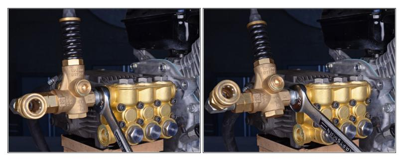
• Use a 3/4" or adjustable wrench to loosen and disconnect the coupling from the pump assembly.
