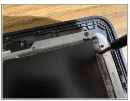
Remove the four M2.5x2 PH#0 screws holding the LCD in the display.
