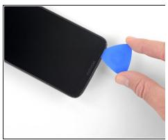
• Slice through the glue under the lower bezel.
