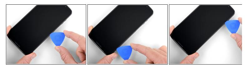
Slide the tool all along the right edge of the phone to slice through the adhesive securing the display.
