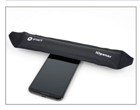
Heat the upper edge of the display to soften the adhesive underneath.
