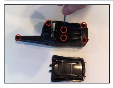
• Unscrew the six 8.0 millimeter long, #0 screws on the backside of the case using the Phillips #0 screwdriver.
