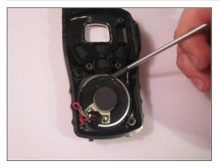
• Scrape off the glue on the outer lining of the speaker using the metal spudger.
