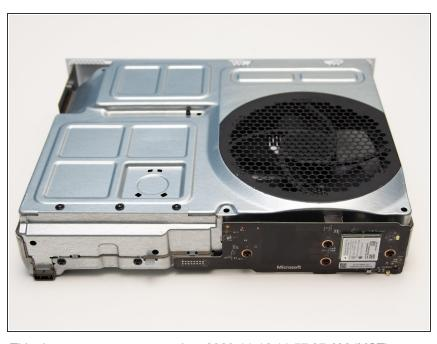
Flip the metal enclosure so that the fan cover is on top. To reassemble your device, follow these instructions in reverse order.
