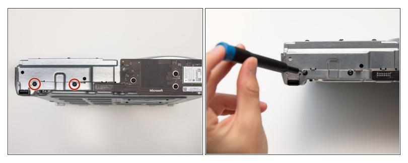
• Remove the two 15mm screws from the front panel using the Torx T8 screwdriver.
