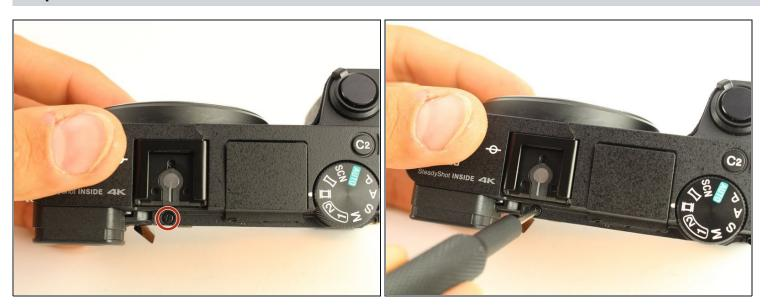
(i) The last screws holding the top on can be accessed once the back of the camera is removed.
