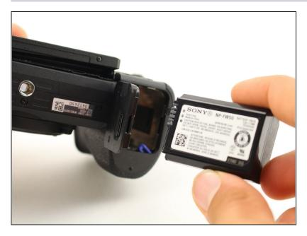
• Remove the released battery from the compartment.
