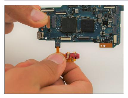
Disconnect the wire ribbon connecting the power port to the board.
