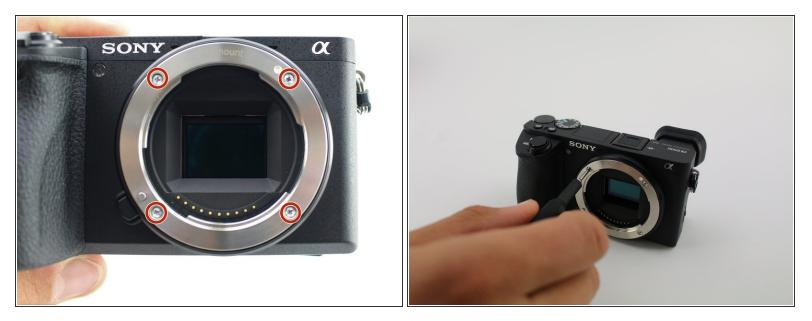
Use a screwdriver to remove four 5mm JIS 00 screws from the lens mount.
