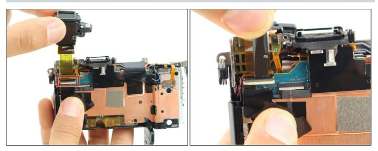
• Lift the viewfinder out and flip up the tab to release the wire ribbon where it is connected to the motherboard.
