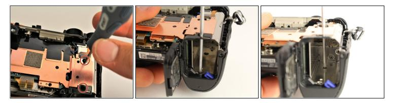
Insert a long, thin JIS 00 screwdriver through the two holes and into the battery compartment; remove the two 5mm JIS 00 screws inside it.
