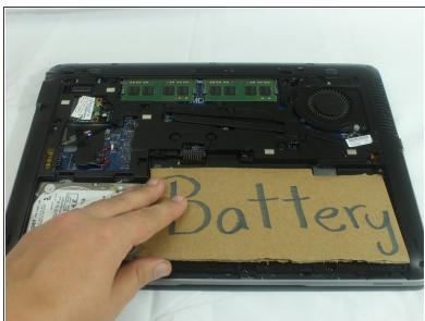
Gently lift up on the battery (represented by this cardboard cutout) until it disconnects. Once the battery is disconnected lift away from laptop.
