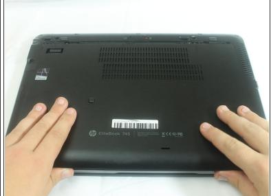
Remove the cover by sliding the lock to the left. You will hear a click once the cover has been unlocked. Gently push down on the cover and slide it towards you to remove it.
