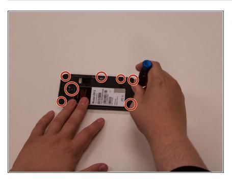
Remove the seven 2mm Phillips #00 screws from the midframe of the device.
