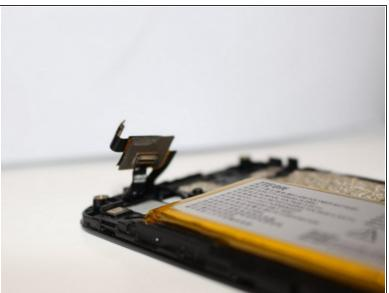
Disconnect the earpiece from the screen with tweezers or a spudger.
