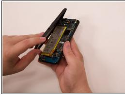
Use an opening tool or fingers to separate the midframe covering the rest of the device starting at the top corner.
