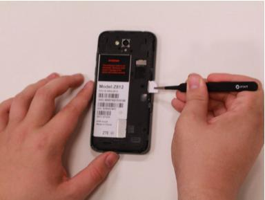
Remove the SIM card from the right side of the device using a pair of tweezers.
