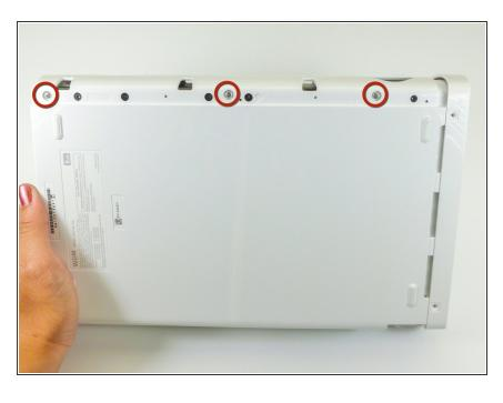
On the bottom of the console beneath the previously removed faceplate, remove the three 13.2mm Tri-wing Y1 screws.
