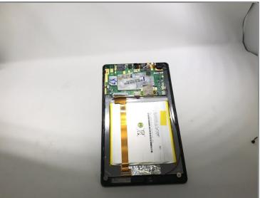
• Remove the silver/metallic tape covering the blue and red wires overlapping the upper and lower end of the ribbon cable.
