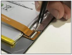
• Remove the ribbon cable by pulling the locking tab of the ZIF connector up and pulling the ribbon cable out with tweezers.
