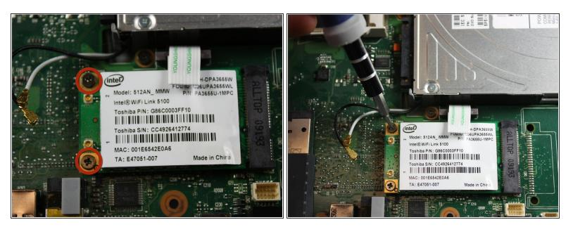
Locate and remove the two Philips #00 4.85 mm screws on the left of the WiFi card.
