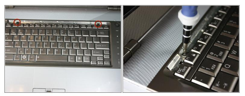
Using your Phillips #00, unscrew the two 4.80mm screws at the top of the keyboard.
