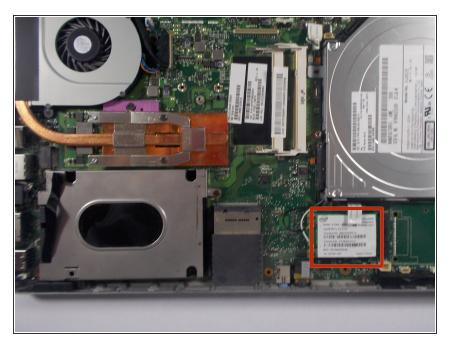
• Locate the WiFi card, which is directly beneath the disc drive.
