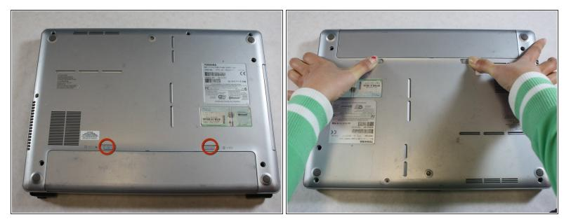
• Slide both of the latches to the outside to release the battery.
