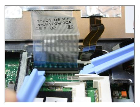
Using the plastic opening tools, pop out the ribbon cable from the rest of the computer.
