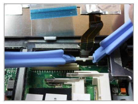
• Using the plastic opening tools, pop out the second ribbon cable from the rest of the computer.
