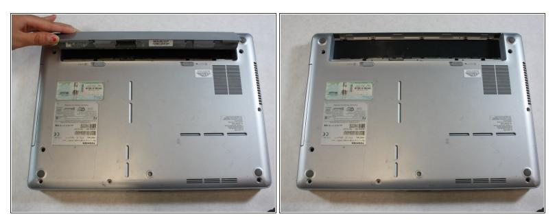
• Pull the battery out by lifting the battery cover away from the laptop.
