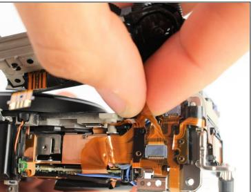
• Carefully unplug the two ribbon connectors attaching the top assembly to the rest of the camera.
