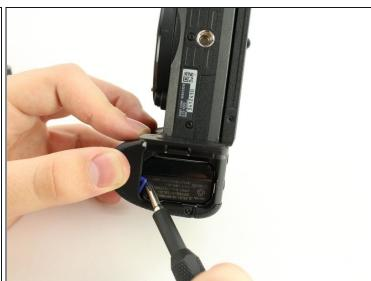
• Push the blue lever aside to release the battery.
