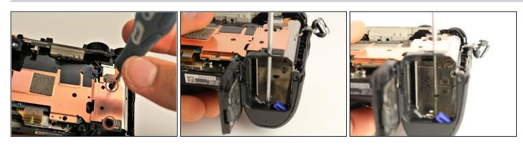
• Insert a long, thin JIS 00 screwdriver through the two holes and into the battery compartment; remove the two 5mm JIS 00 screws inside it.
