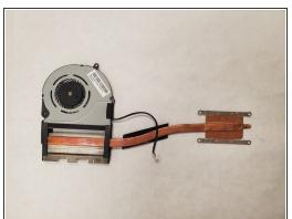
Remove the small, beige colored connector securing the fan to the laptop and remove the fan and heatsink assembly from the laptop.
