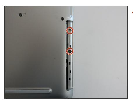
Remove the 3mm screws that were hidden under the Optical Drive with a Phillips #0 screwdriver.
