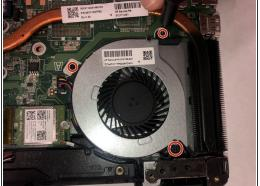
• Remove the three 3mm screws with the Phillips#00 screwdriver.
