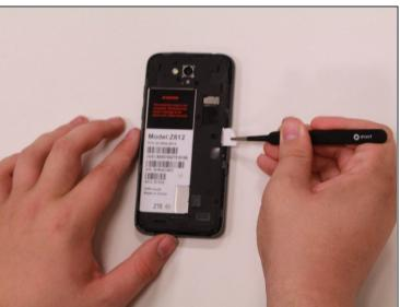
• Remove the SIM card from the right side of the device using a pair of <u>tweezers</u>.
