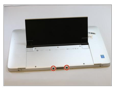
Use a Phillips #00 screwdriver to remove the two 3.5 mm screws from the bottom of the device—one on each side of the keyboard dock.
