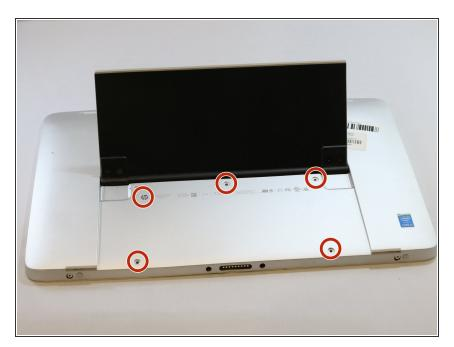
Remove five 4mm Phillips #0 screws securing the lower case to the HP Envy x2 13-j002dx.
