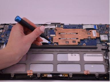
Using a Phillips #0 screwdriver, remove the three 3.8 mm screws along the edge of the motherboard.
