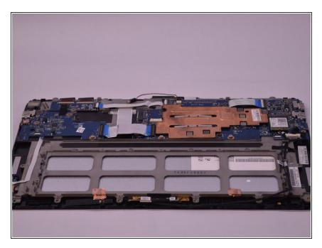
Before removing the motherboard, clear away any dust, and ensure that the battery is already removed.
