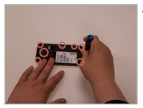
Remove the seven 2mm Phillips #00 screws from the midframe of the device.
