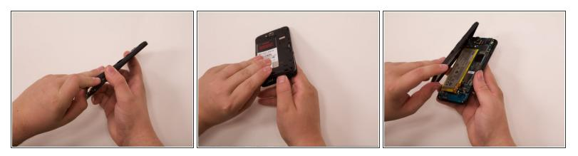
• Use an opening tool or fingers to separate the midframe covering the rest of the device starting at the top corner.
