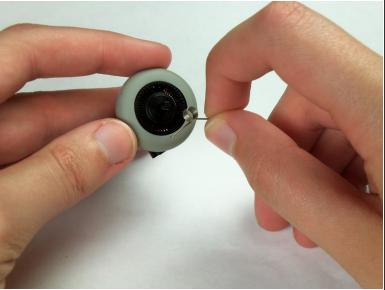
Locate the spring on the scroll wheel, and carefully remove the spring.
