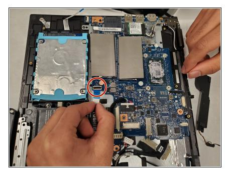
Remove the connector by flipping up the black switch and pulling the blue tipped cable out.
