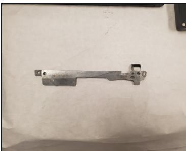
• Using a Phillips #00 screwdriver, remove the two screws on the top left corner of the USB protector (metal bar located on the left side of the motherboard).
