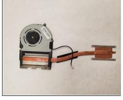
Remove the small, beige colored connector securing the fan to the laptop and remove the fan and heatsink assembly from the laptop.
