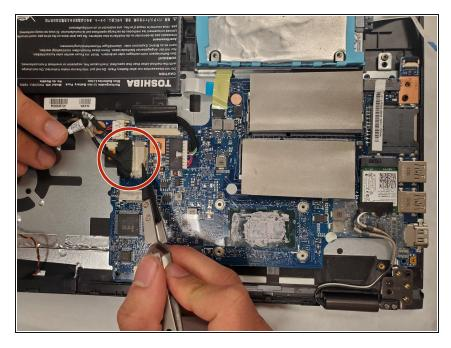
Remove the display cable located directly below the "M/B" cable by removing the tape and pulling the cable to the right while keeping it parallel to the laptop.
