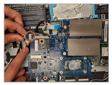
Remove the wireless adapter (white rectangle attached to surface of motherboard).
