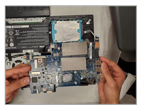
Remove the motherboard from the device.
