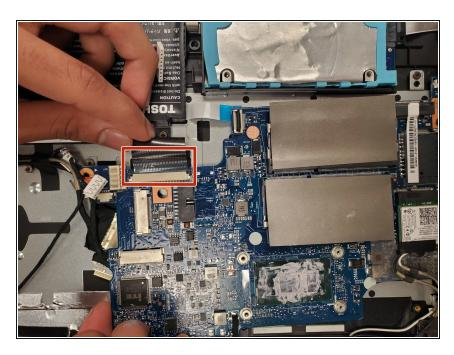
Pull up the black tab located to the left of previously removed connector cable.
