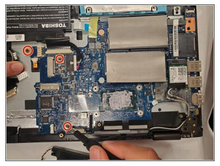
Use the Phillips #00 screwdriver to remove the three screws securing the motherboard to the laptop (located on rectangular/circular copper surfaces).
