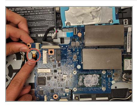
Remove the cable connecting the motherboard to the laptop (located on right side of motherboard).
