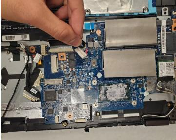
• Remove the second battery connector attached to motherboard (larger of the two).
