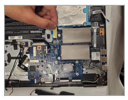
Remove the yellow tape above the battery connector (located above top right corner of hard drive).
