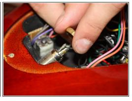
Remove the loosened nut completely by rotating it counter-clockwise.
