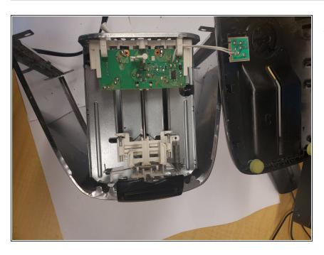
The circuit board is welded to the heated filaments. In order to further open up the toaster frame, this step is necessary.
