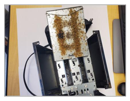
Unlatch bottom crumb collector by removing the metal tab and wires connecting it to the base of the metal structure. This reveals a way to clean the toaster in the future.
