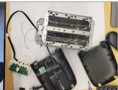
• The spring shown makes the lever bounce back up after the toast is done. The latches hold the toast in place when the lever is down.
