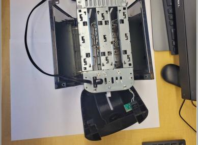
These covers were attached by the four screws at the bottom. To remove them, simply pull up and shimmy them out of their slots. However, the front cover still has electrical attachments.
