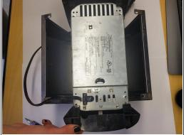
Removing the bottom four screws allows the metal casing to open.
