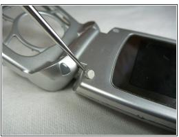
Pry the grey pieces of plastic off the corners of the screen with a spudger.
