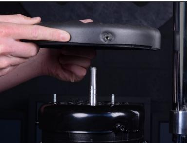
Lift the blower plate up and remove it from the motor assembly.
