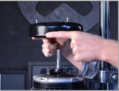
Lift the fan cover and remove it from the motor assembly.
