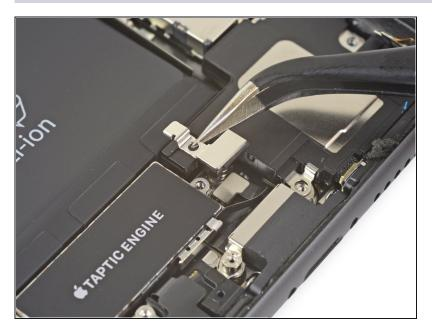
Remove the Taptic Engine connector cover.
