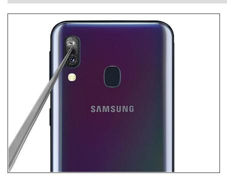
Pull out the little glass shards and be sure not to damage or scratch the camera lenses just underneath.
