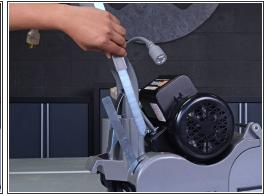
Slide the collar on the control link arm up until the two halves of the arm detach from one another.
