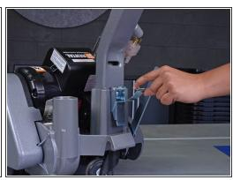
Pull up on the latch at the bottom of the handle assembly, then remove the retaining plate from its slot in the handle.
