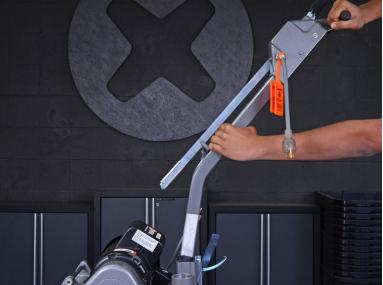
Pull up on the handle assembly and remove it from the sander.
