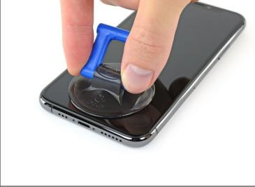
• If you're using a single suction handle, apply it to the bottom edge of the phone, while avoiding the curved portion of the glass.
