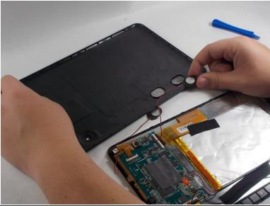
Remove the speakers from the case by gently lifting them up and out of their slots.
