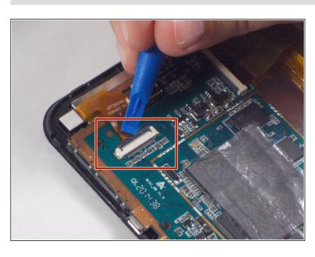
Use your thumb or opening tool to lift the black connector holding in the ribbon cable.
