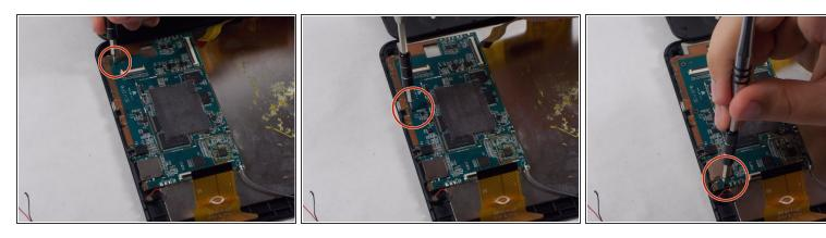
Remove three JIS #0 screws that hold the motherboard to the screen.
