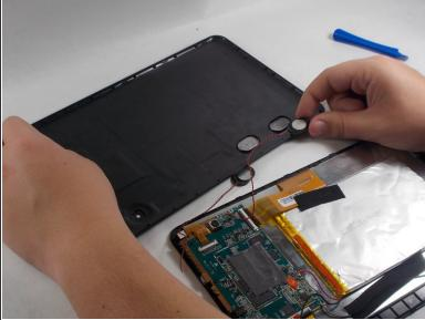
Remove the speakers from the case by gently lifting them up and out of their slots.
