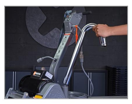
Pull up on the dust tube to remove it from the sander.
