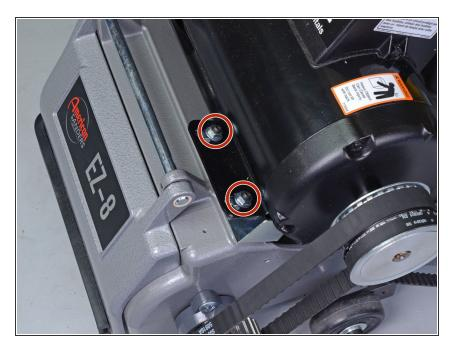
Use a 1/2" wrench to loosen the other two nuts securing the motor.
