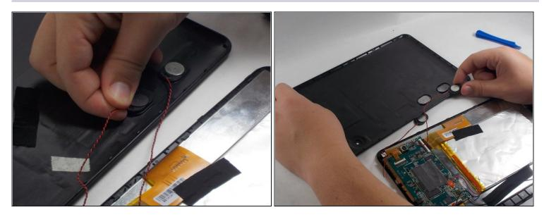
• Remove the speakers from the case by gently lifting them up and out of their slots.
