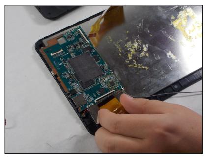
Use your finger to lift the black connectors on each ribbon cable. Remove both ribbon cables that connect the two screens to the motherboard by pulling them out of the connectors.
