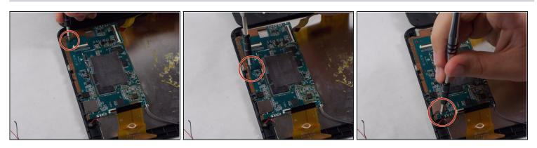
• Remove three JIS #0 screws that hold the motherboard to the screen.
