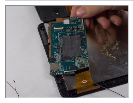
Remove the motherboard by simply lifting it up off the LCD.
