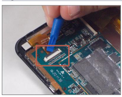
Use your thumb or opening tool to lift the black connector holding in the ribbon cable.
