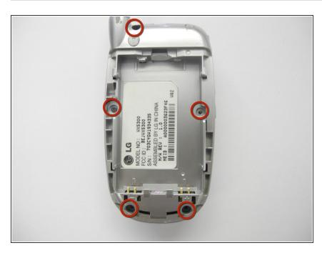
Using a Phillips #0 screwdriver, remove the five screws from the back cover and carefully set them aside.
