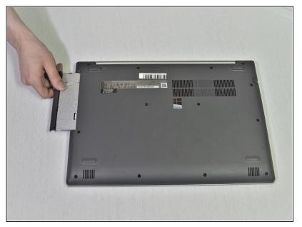
Carefully remove the optical drive by pulling the bezel away from the laptop.
