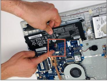
• Pinch the connecting cord with one hand and pry the battery connector with the other hand, while gently pulling the connector straight out and towards the bottom edge of the base.
