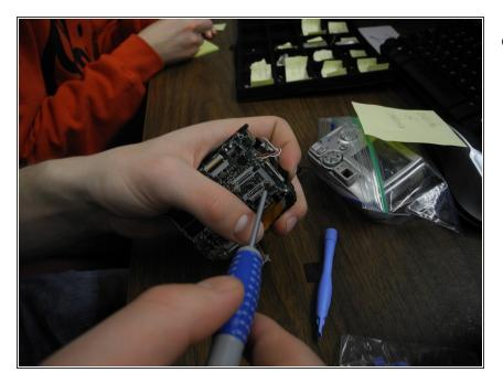
• Unscrew the two screws underneath.
