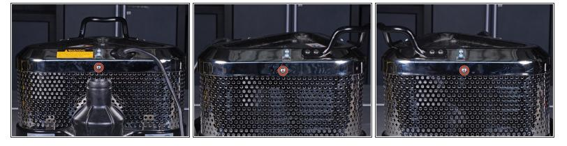
• Use a Phillips #2 driver to remove three 22.1 mm-long screws securing the motor cover to the sander. There is one screw on each side of the sander.
