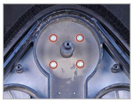
Use an 11 mm socket to remove the four 22.8 mm-long screws securing the motor.
