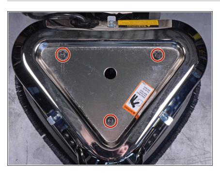
Use a 7/32" hex key to remove three 23.7 mm-long hex screws securing the motors to the motor cover.
