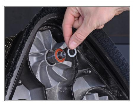
Remove the washer from the motor shaft.
