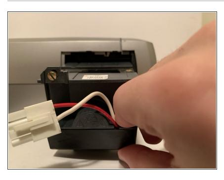
Pull on the bottom plastic tab and remove the lamp by hand.
