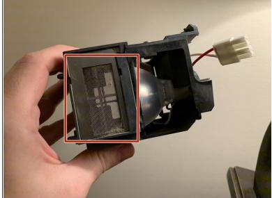
• Use a vacuum cleaner to gently suck up the dust on the front and the back Lamp Housing screens.
