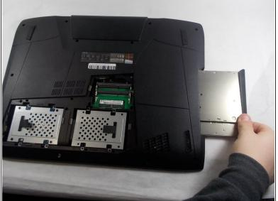
Use a spudger to pry the disc drive out of the laptop.
