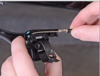
Grab the open end of the throttle cable and pull it out of the throttle lever to free it from its recess.
