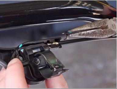
• Use a pair of needle-nose pliers to remove the small clip attached to the throttle cable.
