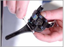
Continue to lift the throttle cable out of the throttle lever, making sure it clears the openings in the recess.
