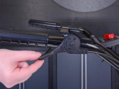
Push the throttle lever all the way down.
