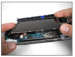
• Push the homebar to the right to release the tab on the right side of the LCD screen.
