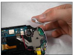
• Unscrew the 'R' trigger and remove both pieces. (Refer to step nine by applying the procedures to this, the right, side)
