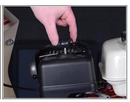
Use your fingers to unscrew and remove the wing nut securing the air filter cover.
