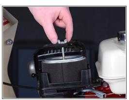
• Use your fingers to unscrew and remove the wing nut securing the air filter.
