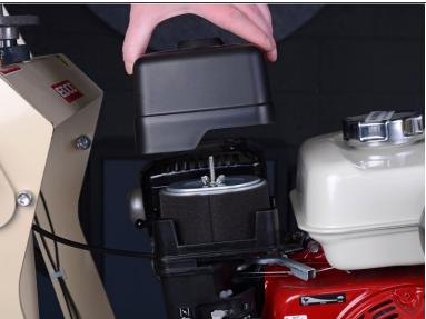
Lift the air filter cover straight up to remove it.
