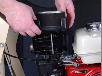
Grab the black plastic air filter platform and lift it straight up with the air filter to remove both components.
