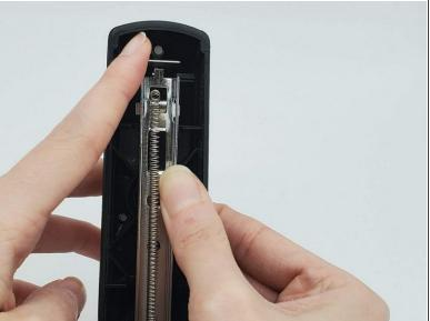
Push the hammer, the rectangular piece, up and away from the metal part.
