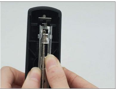
Press the metal part down with your thumbs until it aligns with the hammer's hole.
