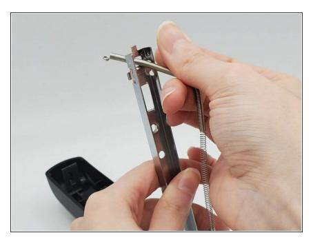
Thread the other end of the new spring through the top rectangular hole toward the back.
