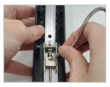
Hook one end of the new spring onto the pusher's hook.
