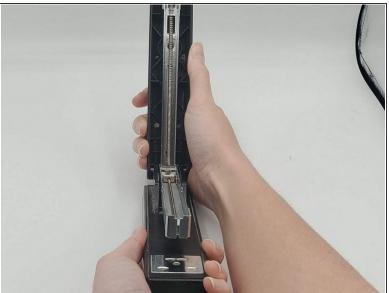
Open the stapler by gripping the handle to access the spring.
