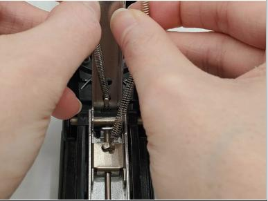
Hook the new spring to the hook on the inside of the handle's metal part.
