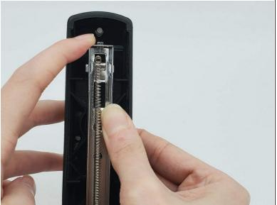
Reattach the hammer back onto the metal part.
